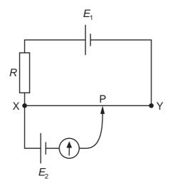
The circuit is changed so that the galvanometer reads zero when the sliding contact is at a new position to the left of P.
