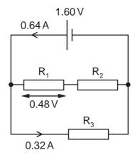
The cell has electromotive force (e.m.f.)  $1.60\,\mathrm{V}$  and negligible internal resistance. The current in the cell is  $0.64\,\mathrm{A}$ .
